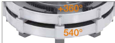
The Innovation is a heavy-duty jack-up vessel for installing and maintaining offshore wind farms. The igus® multi-rotation module is the main power supply for the crane which operates around the leg. The 2 layer design allows a rotation angle of 900°.
