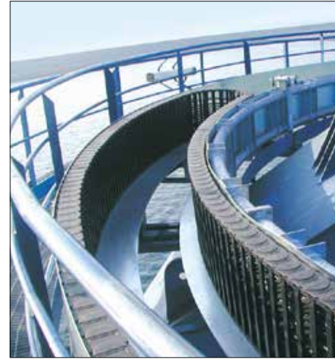
Opposing series 5050 e-chains® with igus® guide trough system and support structure – outer diameter: 12 m, rotation angle: 340°.
