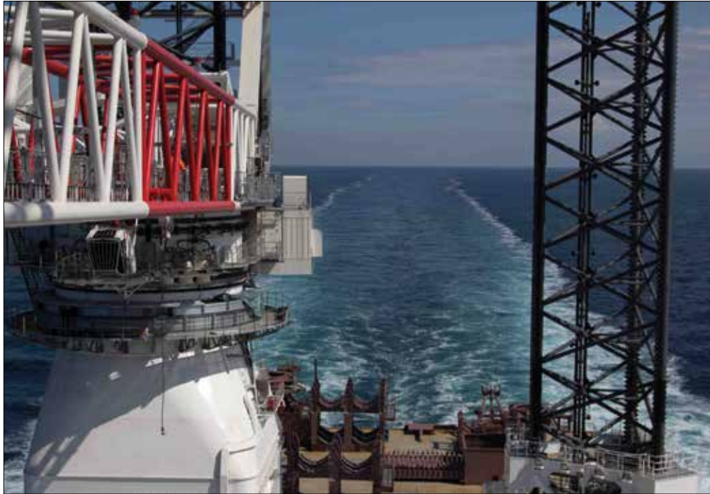
The Innovation is a heavy-duty jack-up vessel for installing and maintaining offshore wind farms. The igus® multi-rotation module is the main power supply for the crane which operates around the leg. The 2 layer design allows a rotation angle of 900°.
