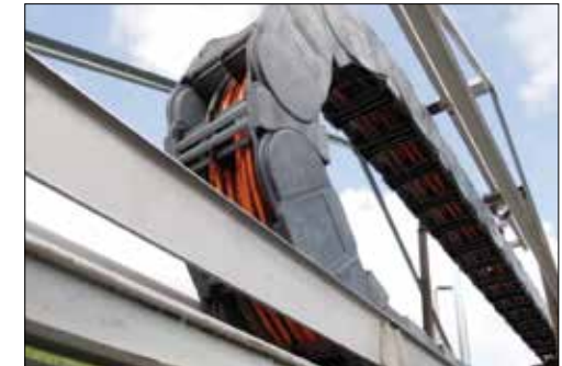
E4.350 to be installed on a skidding application on an FPSO. Stainless steel guide trough with hook attachment.
