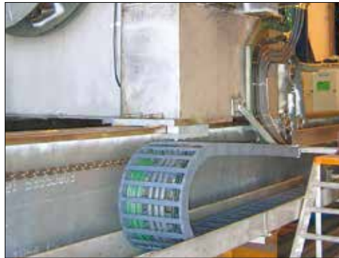
ATEX version of the igus® e-chainsystem®, series E4, harnessed with hydraulic hoses and igus® chainflex® cables. Here shown on a test stand, now in operation on the Dalia FPSO (linear motion of mooring).
