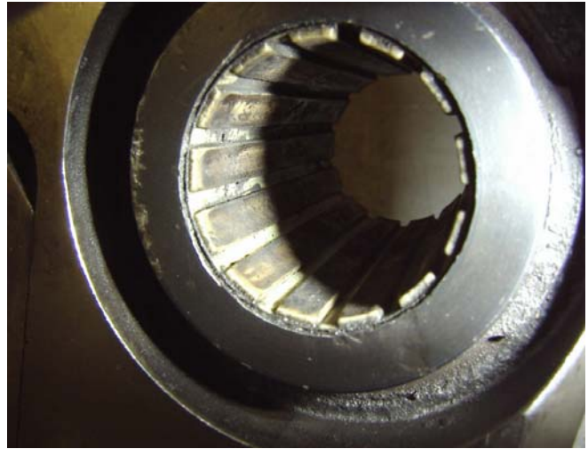
Picture PM2905-04: igus GmbH, Cologne Linear guide with high-performance polymer sliding element.
