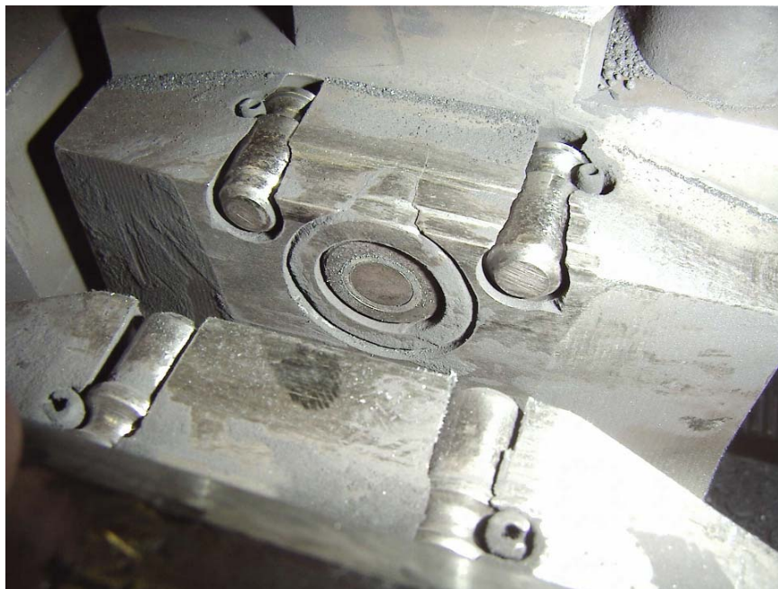
Picture PM2905-01: igus GmbH, Cologne Ejectors, guided on self-lubricating "DryLin R" bearings from igus.
