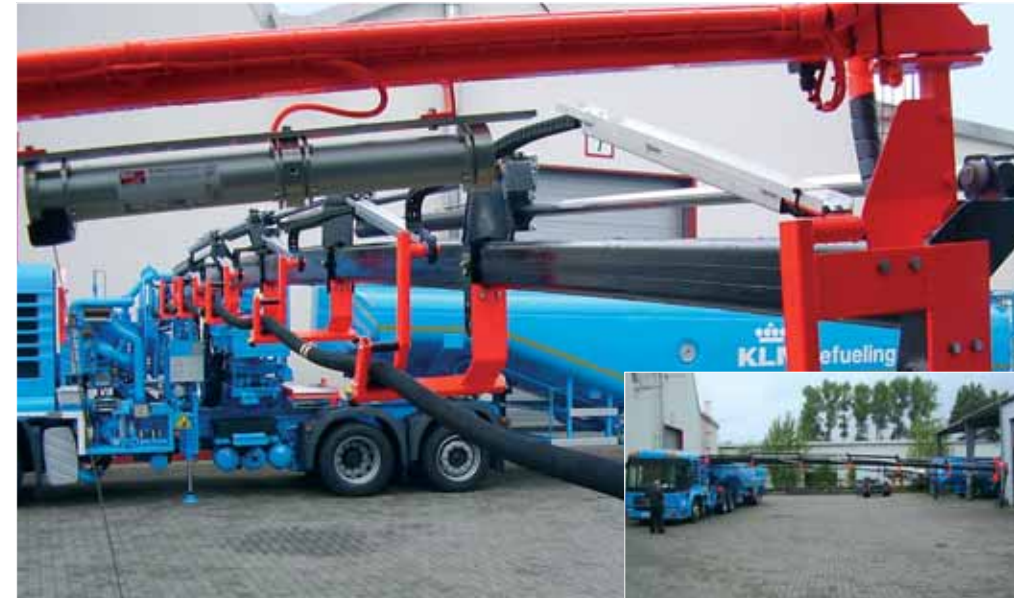
E2/000 Series 1400 in aircraft refueling truck; telescopic crane with six sections
