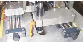
Positioning of cutter heads with DryLin® SHT-20-SWM, Berchtold GmbH, Germany
