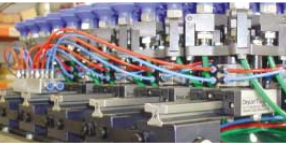
DryLin® T in tile handling system, Kautenburger, Merzig, Germany
