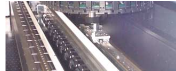
DryLin® W in flatbed inkjet printer, Durst Phototechnik
