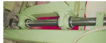
DryLin® R in concrete pipe cutter, Haas Maschinenbau, Oberbrück
