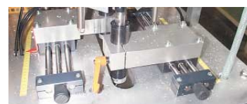
Positioning of cutter head with DryLin® SHT-20-SWM, Berchtold GmbH
