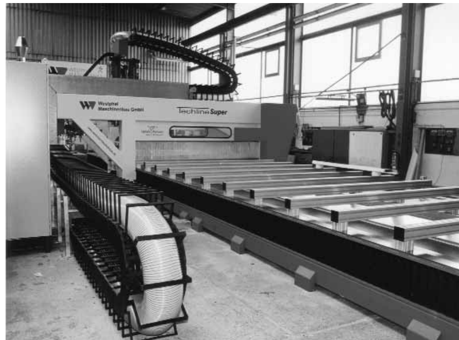
igus® E-Chain® with extender-crossbar - safe guide for big hoses
