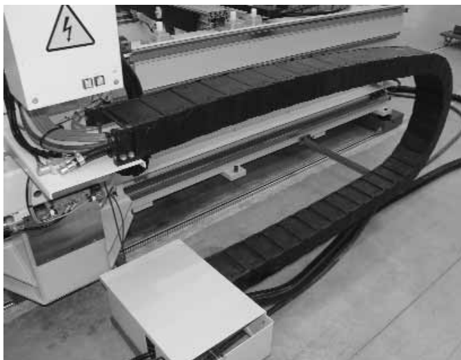
E4/light E-Tubes protect tubes and hoses safely against dirt and chips
