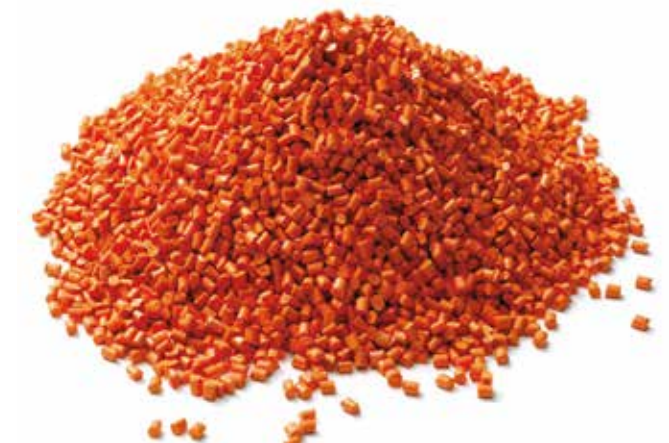
Picture 05: Polymer granulate, basis compound of the lubrication-free and predictable iglidur® bearings
