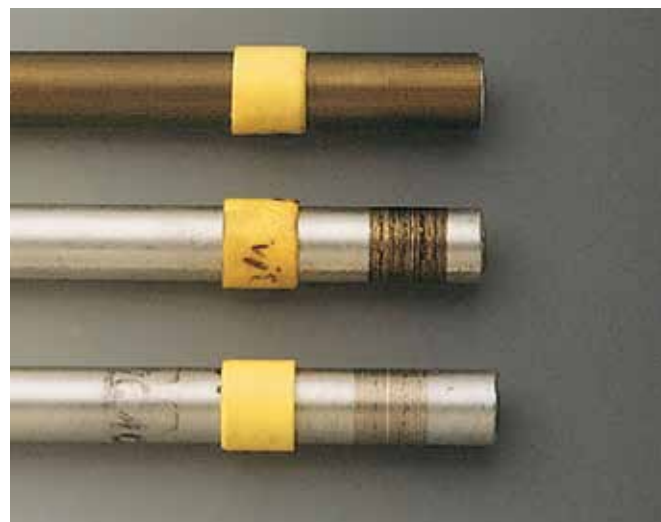
Picture 10: Wear experiments with aluminum shafts
