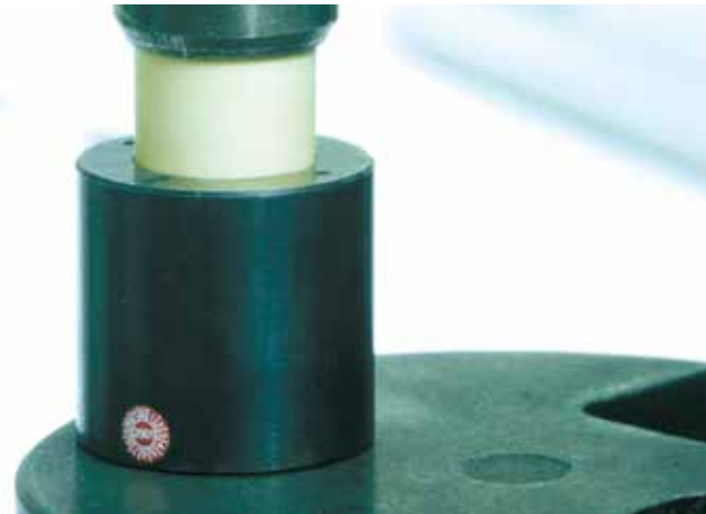
Picture 15: The bearing should be press fitted using a flat press.
