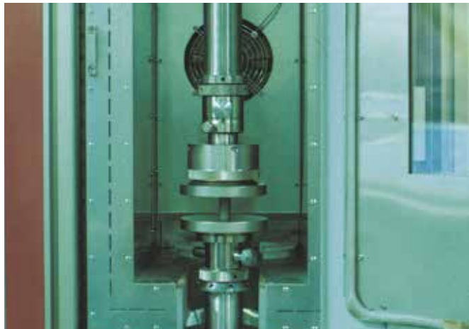
Picture 08: Material tests are possible up to +250 °C
