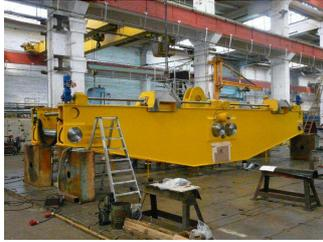
*Fig 2: The heavy-duty shaft end support allows the flexible positioning of all four winches or attachment points.*
